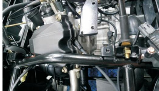
*Spark plug cap, front cylinder*
